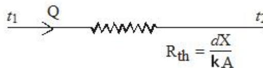
$$\text{Heat flow } q = \frac{\text{Temperature difference } (dt)}{\frac{dX}{kA}}$$
