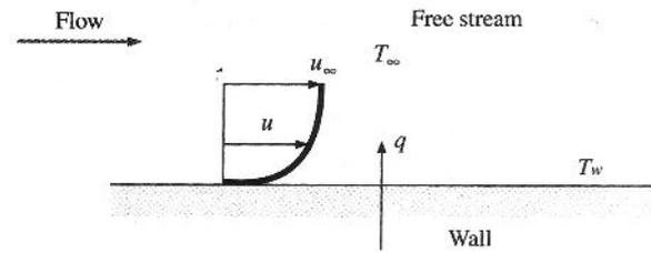
**Figure-2: convection heat transfer from a plate.**
